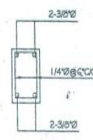
DETAIL "C" BEAM 6" X 12"
